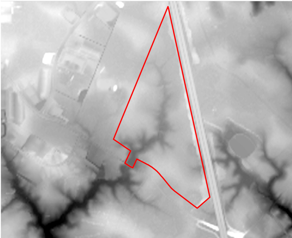
Figure 5 – Digital Elevation Model. The red line depicts the approximate Site boundaries. The darker indentations show lower elevations and the lighter colors are higher elevations. The red property boundary is the only addition to the depiction.
